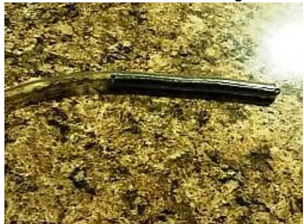
Lead tool inserted in tubing
